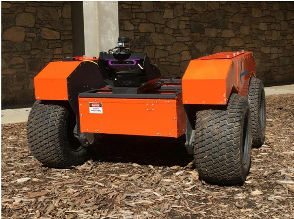
A Canadian company that develops all-terrain robots to explore the Moon has adapted its technology and builds robots for farming. The result is a mobile platform called Argo J5 XTR (above). The platform is already used to spray banana plantations in the Caribbean. Before using this robot, agricultural workers were exposed to fungicides, rough terrain, and high temperatures during the day. The robot can be remotely controlled by an operator more comfortably and safely.
