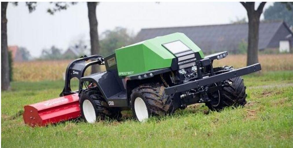
Greenbot is an autonomous tractor (above) that uses a diesel engine to generate power. It is guided by GPS and has software specially designed to be used by the operator for commands and data analysis. The tractor robot comes with a series of systems for detecting obstacles, animals, people, etc. In front, it has mounted a radar and a bumper bar with mobile parts to detect the impact. Additionally, in the bumper are installed other sensors for detection.
