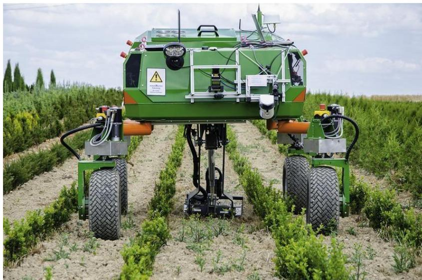
The new BoniRob robot (above) is capable of distinguishing between weeds and crops by comparing them to images using machine learning.
